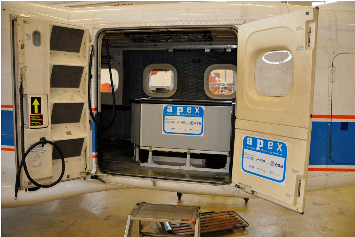
Image 3 - APEX (Airborne Prism Experiment) installed in DLR's Dornier DO-228 research aircraft pictured just before a data take (Photo: APEX Team).
