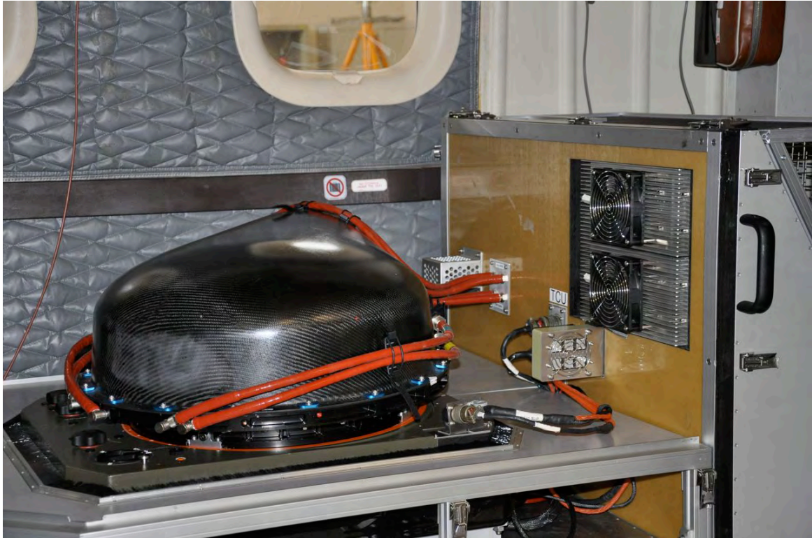
Image 2 – APEX (Airborne Prism Experiment) installed in DLR's Dornier DO-228 research aircraft. The black cover comprises the spectrometer part of APEX, and the gray box to the right holds the climate control unit of APEX (Photo: APEX Team).
