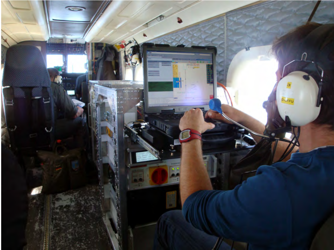
Image 6 – APEX operation during data acquisition. The operator (right) is equipped with an oxygen mask for high altitude flights. The rack in front of the operator is used to steer data acquisition (Photo: APEX Team).
